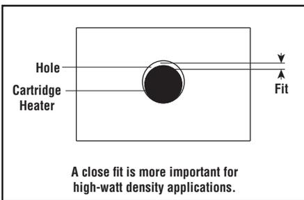
**Determining Watt Density** — Watt density refers to the heat flow rate or surface loading. It is the number of watts per square inch of heated surface area. For calculation purposes, CIR stock cartridge heaters have 1/4" unheated length at each end. Thus, for a 1/2 x 12" heater rated 1,000 watts, the watt density calculation would be as follows:
