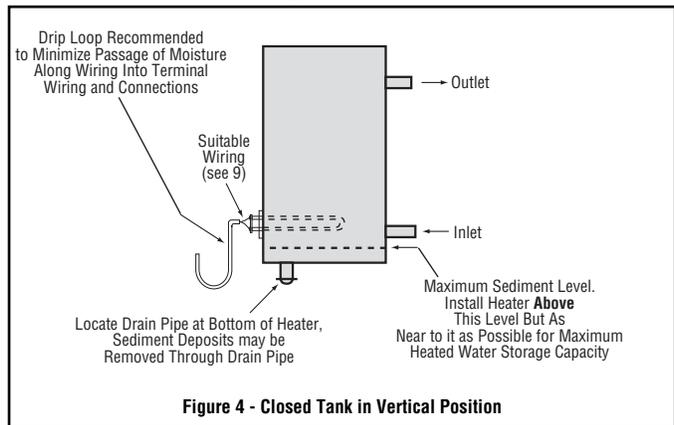
9. **WARNING: Hazard of Electrical Shock. Exposed electrical terminals must be properly guarded to prevent electrical shock.**
