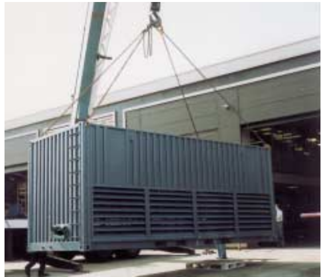
Containerized 3.5 MW load bank.
