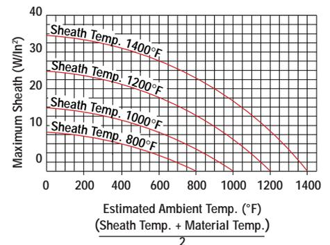
The example on the following page illustrates the procedure. 12 kW is required to heat material in a steel tank from 70°F to 800°F. Heat is to be supplied by tubular electric elements clamped to the side of the tank. Since the material is heated to 800°F, INCOLOY® sheath elements must be used.
