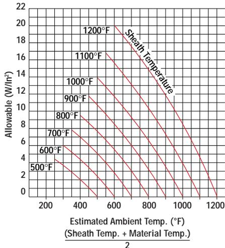
Using the previous 12 kW example, determine the number of strip heaters required. An 800°F material temperature requires chrome steel strip heaters. From Graph G-130S, a maximum sheath temperature of 1200°F results in an ambient temperature of 1000°F inside the space between the thermal insulation and the vessel,  $(800^{\circ}\text{F} + 1200^{\circ}\text{F}) \div 2 = 1000^{\circ}\text{F}$ .
