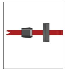
Using standard electrical cutters, cut a "VEE" notch between the buss wires.
