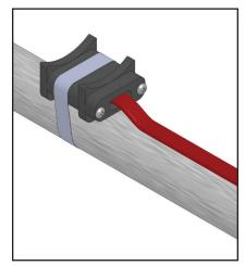
6. Using a fastening device, fiber reinforced electrical tape (Chromalox FT-3 or equal), secure the assembly to the pipe. Wrap the tape around the assembly between the legs.
