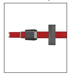
Score the outer jacket one inch from the end of the cable. Remove the jacket to expose the braid. Unravel and trim the braid flush with the outer jacket. Pull any strands of braid back towards the outer jacket.
