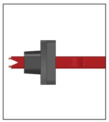
4. Slide the pressure plate and grommet towards the end of the cable leaving 5/8" of the cable past the end of the grommet.
