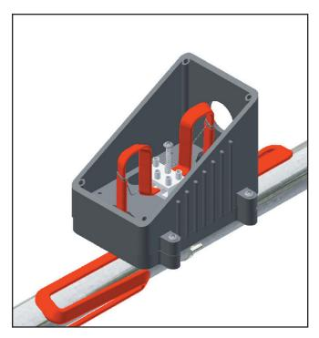
Mount terminal block to bottom of the box by driving the self-tapping screw (Item 8) provided into the mounting hole as shown.
