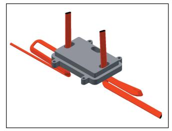
Feed the ends of the cables through the appropriate hole in the base. Allow 8" of cable to extend above the top of the base.
