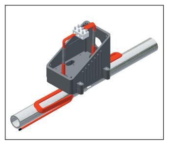
8. Insert the bared ends of the conductors and the braid into the openings in the terminal block. Tighten screws firmly to hold the wires and braid in place.
