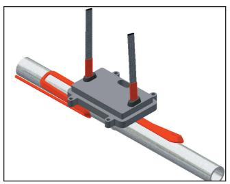
4. Score the outer insulation 7" from the end of the cables. Remove the jacket to expose the metal braid. **CAUTION: When removing outer jacket, be careful not to damage the braid of the base cable insulation.**
