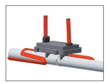
3. Slide cable grommets over the end of the cables and insert it into the opening in the base. Secure the base to the pipe by threading the appropriate sized pipe strap through the slot in the mounting plate. Tighten the pipe strap until the base is securely attached to the pipe.
