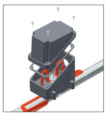
10. Carefully push all the wires into the box and secure the lid to the box. Make sure water tight rubber gasket (Item 5) is in place.
