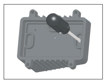
Use a hammer and screwdriver to punch out the knockouts on the bottom of the box which correspond to the openings in the base through which the heating cable passes. Only punch out the knockouts that are to be used. If one is mistakenly punched, blank grommets can be ordered to reestablish the water tight seal.
