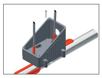
Feed cables through the corresponding holes in the box and secure box to base using all four of the 1" long screws (Item 11).
