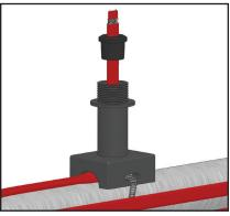
Using wire cutters trim exposed grounding braid away from the end of the cable.
