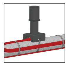
6. Tighten end cap until it bottoms out on pipe standoff.
