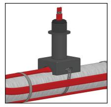
4. Adjust cable leaving 1" past the end of the grommet and in sert the grommet into the pipe standoff. Attach extra cable to pipe as shown.
