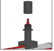
Slide end cap over cable. Grom met should be placed inside pipe standoff.
