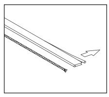
7. Starting at the end of the heating cable, using needle nose pliers or a knife pull each bus wire away from the core material. \*Separate CWM-C leads and strip 1/4" from each leadwire.
