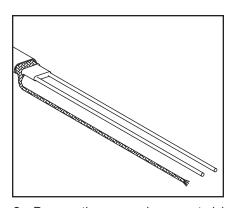
Remove the exposed core material and cut 1/4" of the end of each bus wire. \*Skip this step if using CWM-C constant wattage cable.
