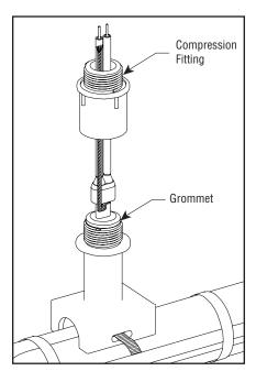
10. Slide compression fitting over cable. Grommet should be placed inside pipe standoff. Termination boot should be spaced 1/2" from sealing grommet.
