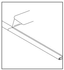
4. Score the inner insulation 7" from the end. Lightly cut the inner jacket up the center to end of heating cable and remove the inner jacket from the cable.
