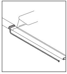
5. Score the inner insulation 6" from the end. Lightly cut the inner jacket up the center to end of heating cable and remove the inner jacket from the cable.
