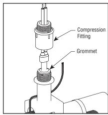
Slide compression fitting over cable. Grommet should be placed inside pipe standoff. Termination boot should be spaced 1/2" from sealing grommet. Tighten compression fitting until it bottoms out against pipe standoff.
