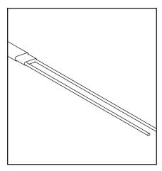
Remove the exposed core material and cut 1/4" off the end of each bus wire. \*Skip this step if using CWM-C constant wattage cable.
