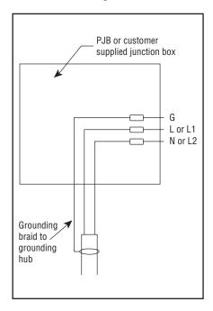
12. Attach conduit hub (Chromalox CCH-2 or equivalent not included) as needed. Using crimp connectors supply power electrical connections should be as shown.
