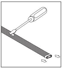
Push braiding back from the end of the cable. 11" from cable end create a bulge. At the bulge, separate the braid to make an opening.
