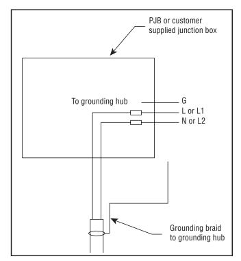
**11.** Attach conduit hub (Chromalox CCH-2 or equivalent not included) as needed. Supply power electrical connections should be brought into box as shown.
