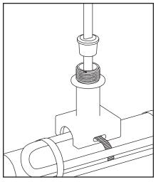
1. Insert heating cable through pipe standoff and grommet as shown. 8" of cable should extend past the grommet. Strap pipe standoff to pipe with pipe strap (Chromalox type PS not included) and attach extra cable to pipe as appropriate. For pipes smaller than 1-1/2" diameter a small pipe adapter (Chromalox model SPA not included) is required.
