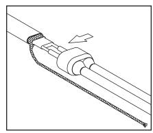
Liberally apply RTV over the exposed matrix and leads. Push the rubber boot over the heating cable. Trim lead ends as needed. \*Boot is not needed when using CWMC constant wattage cable.
