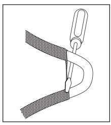
2. While bending the heating cable, work the cable through the braid opening. Pull the braid tight.
