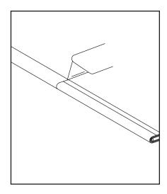
2. Score the outer insulation 7" from the end of the cable. Lightly cut the outer jacket up the center to the end of heating cable and remove the outer jacket from the cable.
