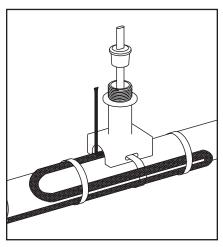
Insert cable though pipe standoff and grommet as shown. Leave braid outside of pipe standoff for future connection to ground. Attach standoff.
