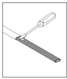
Move braid back toward the overjacket, creating a bulge. At the bulge, separate the braid to make an opening.
