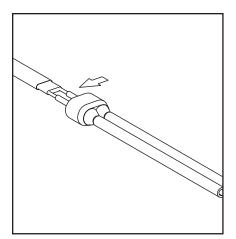
8. Liberally apply RTV over the exposed matrix and leads. Push the rubber boot over the heating cable. Slide cable wires through plastic guide tubes. After boot is in place remove guide tubes and discard. Trim lead ends as needed.
