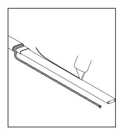
Shave the core material from the outside of each bus wire. \*Skip this step if using CWM-C constant wattage cable.
