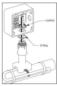
11. Attach junction box to compression fitting as shown. Tighten locknut until the junction box bottoms out against the lip of the compression fitting. The SSK kit is provided with a sealing oring and locknut to attach the compression fitting to a customer supplied junction box through a hole cutout sized 1.313 diameter. Alternately the compression fitting may be threaded directly into a 1" hub.
