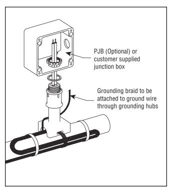
10. Attach junction box to compression fittingas shown. Tighten locknut until the junction box bottoms out against the lip of the compression fitting. The SSK kit is provided with a sealing o-ring and locknut to attach the compression fitting to a customer supplied junction box through a hole cutout sized 1.313" diameter. Alternately the compression fitting may be threaded directly into a 1" hub.
