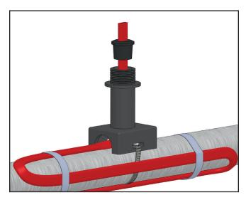
1. Insert heating cable through pipe standoff and grommet as shown. 1-1/2 Inches of cable should extend past the grommet. Strap pipe standoff to pipe with pipe strap (Chromalox type PS not included, UESL to be moiunted vertically only) and attach extra cable to pipe as appropriate. For pipes smaller than 1-1/2" diameter a small pipe adapter (Chromalox model SPA not included) is required.
