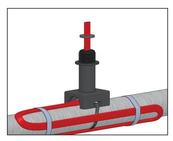
**2.** Place strain relief part onto cable until it is directly on top of the grommet.
