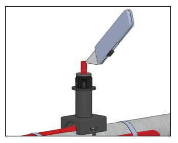
3. 1-1/4 Inches of cable should extend above the grommet. Score the outer insulation 1" from the end of the cable. Lightly cut the outer jacket up the center to end of heating cable and remove the jacket from the cable.
