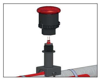
8. Attach LED Assembly to pipe stand off as shown. Liberally apply RTV over the exposed matrix and leads.
