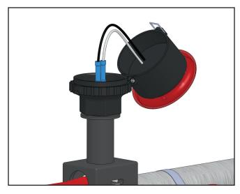
**9.** Using crimping tool crimp white wire from LED assembly to one buss wire and black wire to the other buss wire.
