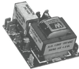
**Note** — For single probe auxiliary low water cutoff (shown with plug-in control relay).
